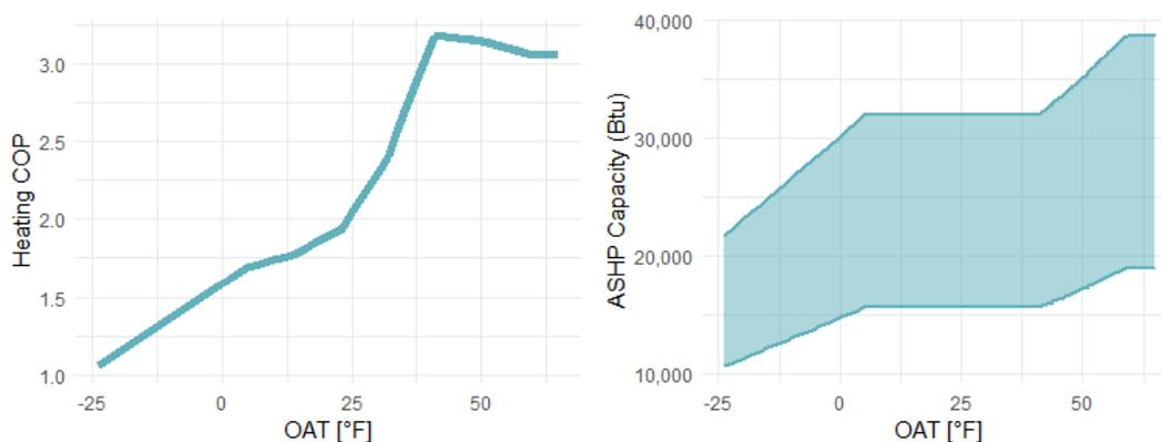
Figure 7: Cold-climate variable speed ASHP performance across heating OATs
