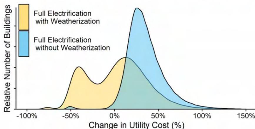
Figure 4: Homes that are not weatherized generally experience cost increases post-electrification, whereas weatherized homes have a broader range of possible cost outcomes<sup>15</sup>
