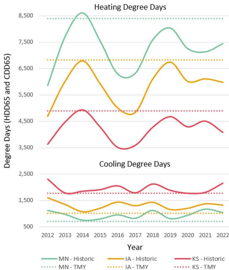
Figure 8: Comparison of historic degree days vs. TMY data for three example climates
